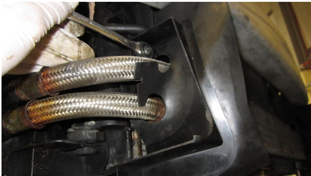
14. There are two final 10mm nuts tucked away behind the plastic cowl to remove. The other 10mm can be found in the same place but on the opposite side.
